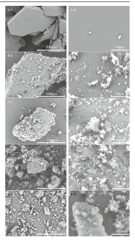
magnification were taken to visualise the effect of milling on the surface disorder or presence of fine particles (<1-2  $\mu m)$  (which is postulated to be amorphous) on the particulate surface (Fig. 3a-ii to e-ii). Fig. 3a-i and a-ii show the un-milled mefenamic acid crystals obtained
