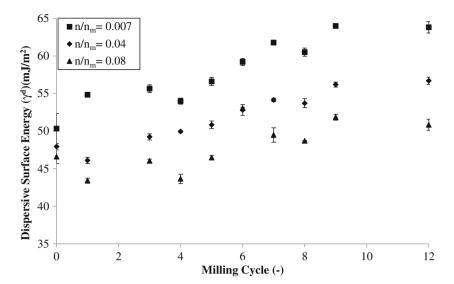
Figure 1 suggests that the surface energy heterogeneity increases post milling, *i.e.*  $\gamma^{\rm d}$  for mefenamic acid recrystallised from methanol, before milling, ranges from 50.3 mJ/m² to 46.6 mJ/m² with varying fractional surface coverage (n/n<sub>m</sub>) from 0.7 to 10% and after one milling cycle  $\gamma^{\rm d}$  for mefenamic acid powder varies from 54.6 mJ/m² to 43.3 mJ/m².
